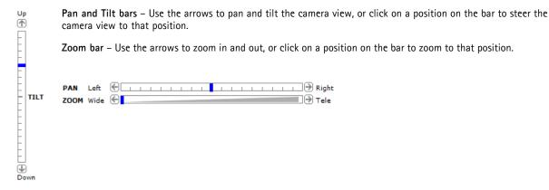
The PTZ controls can be disabled under PTZ > Advanced > Controls, see Controls, on page 28.
